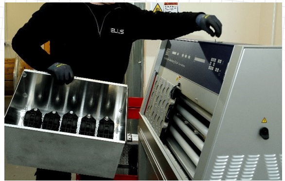
ELLIS' IN HOUSE UV WEATHERING TEST STATION
