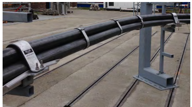
A photo of the short circuit test rig for Centaur Trefoil including Flexi-Straps (see page 26). Testing was carried out at ZKU Laboratories in Prague, CZ.
