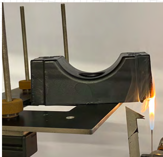
FLAME PROPAGATION TEST ON SOLUS NON-METALLIC CLEAT.
